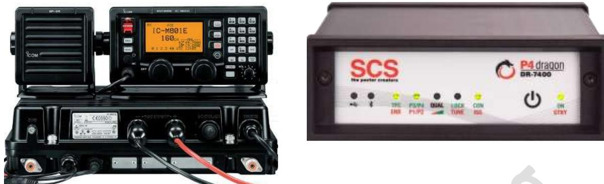
Figure 2 SSB Comms and Pactor Modem
